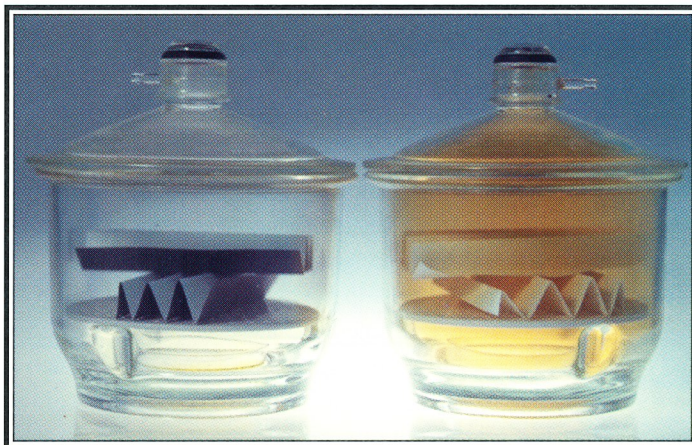
Figure 4. Left, before testing. Right, after one hour, no gas cloud formed in the MicroChamber jar.
